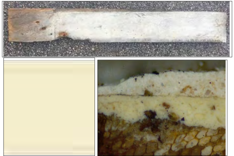
Original painted board from Ailey Young House (top), Benjamin Moore Linen Sand Color Match for Original Paint (bottom left), microscopic slide showing layers of dirt at the bottom, pale yellow in the middle, and white on the top (bottom right).
