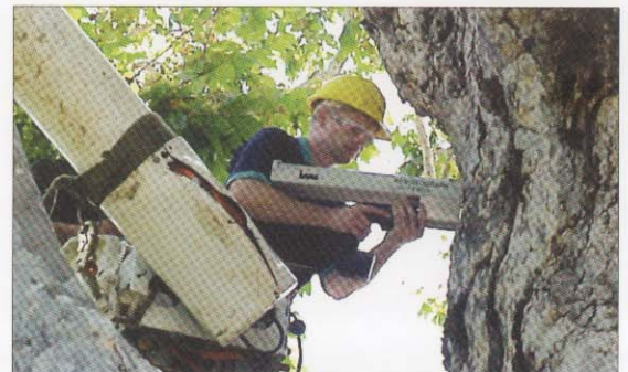
Drilling into a sycamore with a Resistograph.
