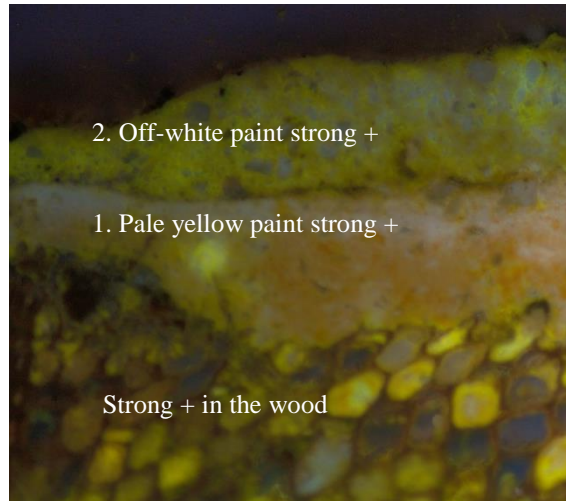
B-2A filter & Alexafluor 488 for proteins 100X No reactions for proteins
