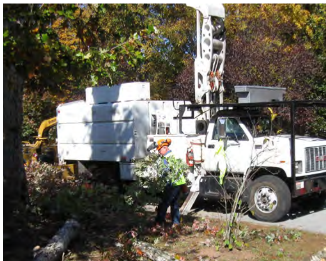
Qualified staff and equipment, such as this bucket truck and chipper, are needed for large tree removal.
