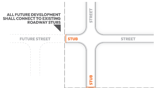
Figure 2: Roadway Stub Location and Arrangement
