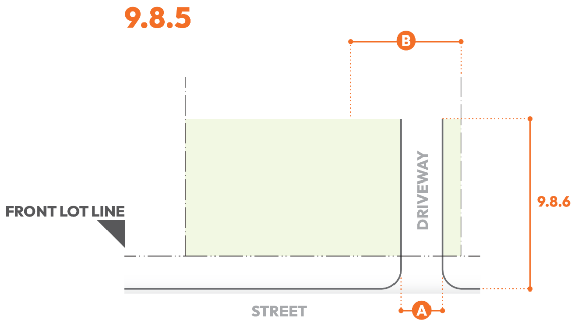
Figure 22: Driveway Width and Length Standards
